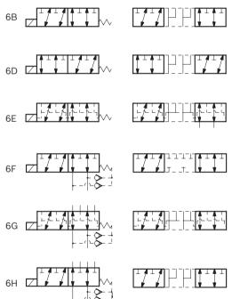
1) Minimum pressure 4 bar (58psi) with external drain (E), maximum pressure 200 bar (2901psi). With internal drain (I), at the minimum pressure (4 bar - 58psi), add the working pressure with ratio of 6,5:1. Example: With working pressure 100 bar (1450psi), minimum pilot pressure is 19.38 bar (281psi) ((100:6,5) + 4 bar (58psi)).
