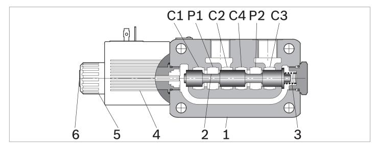
A valve basically consists of a housing (1), a control spool (2), a return spring (3) and a solenoid (5). It is designed to connect two inlet lines P1 – P2 (normally a set of hoses) and divert them to either the outlet ports (C1 - C4) with spool in position "0", when the solenoid is de-energized, or to the outlet ports (C2 - C3) with spool in position "1", when the solenoid is energized.
