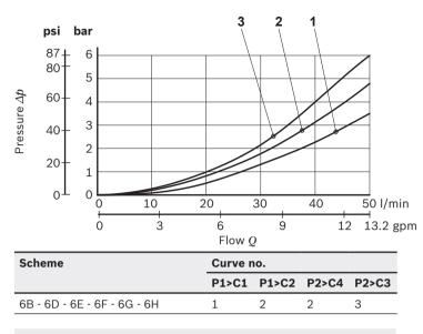
Measured with hydraulic fluid ISO-VG32 at 45° ±5 °C (113° ±9 °F); ambient temperature 20 °C (68 °F).
